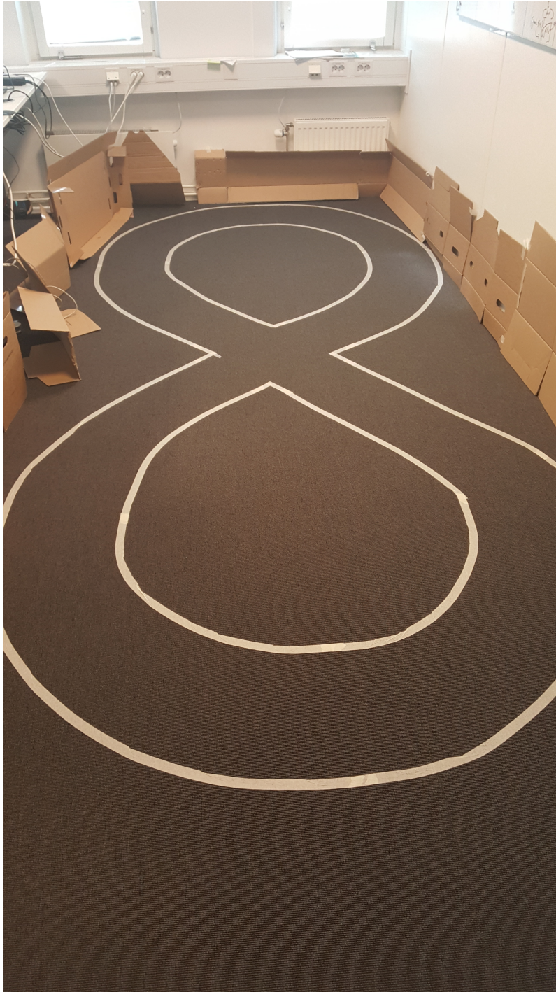
Figure 4.5: The eight track in which the general driving model was trained. The lane width of the track is 35cm.
